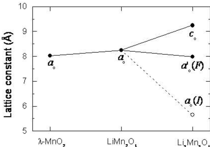
16% change in c/a ratio upon cubic to tetragonal transformation if unconstrained bulk phase
