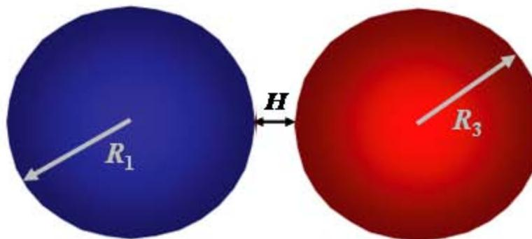
**Interparticle Force Law:**  $F_{vdW} = -\frac{A_{123} R_1 R_3}{6 H^2 (R_1 + R_3)}$
