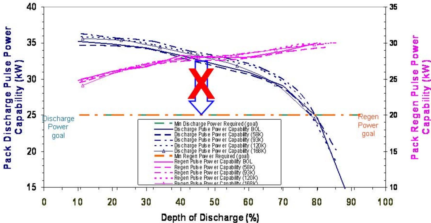
In typical systems, curves shift down due to impedance growth
