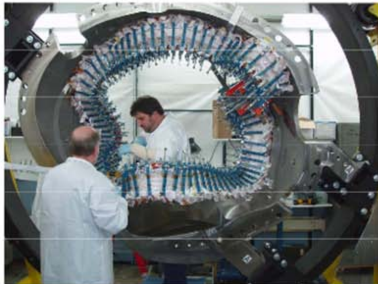
Coil-winding facility 16 of 18 wound.
