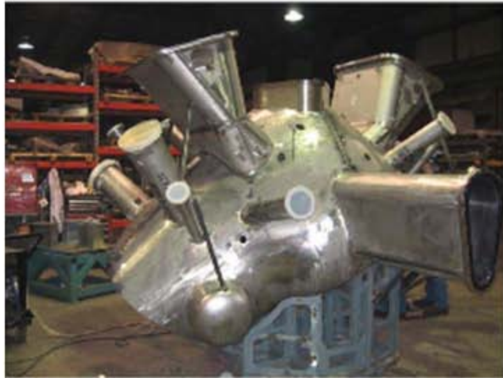
Vacuum vessel All 3 sectors delivered.
