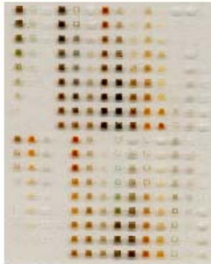
FTO slide printed with binary combinations of eight metals, pyrolyzed to form mixed metal oxides.
